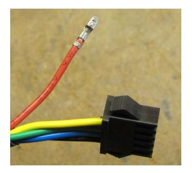
Press down the tab on the opposite side. The tabs should be firmly locked against the wire.
