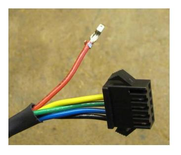
Line up the new contact so that the lower set of tabs is positioned around the wire insulation, and the upper set of tabs is positioned around the exposed wire. Use needlenose pliers to press down one of the tabs.
