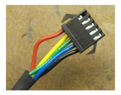
Push the contact into the plastic housing. If it doesn't slide in easily, pull it back out and round up the crimped section some more.
